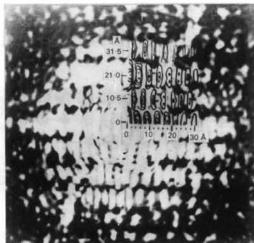
Fig. 13. Two-dimensional cylindrical Patterson function Q(r,z) of EAAC obtained by the optical diffraction method. Solid lines indicate the calculated Q(r,z) .
